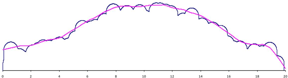
**Figure 5: Particle train and sampling line for a DEM heap (size = 1 reduced unit)**
