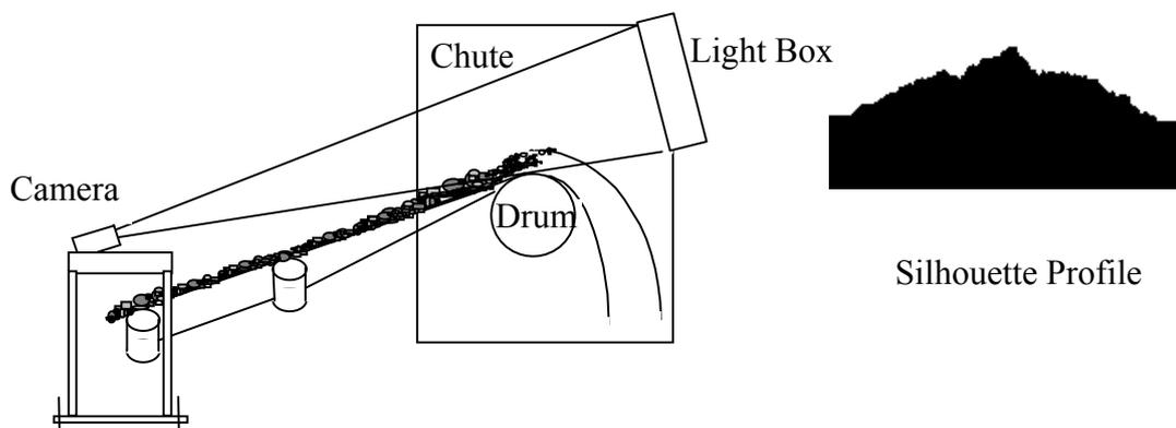
Figure 1: Profile Image Capture at the Head-Drum of a Conveyor
