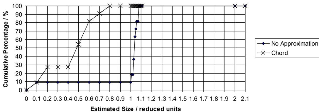
**Figure 9** Size curve showing the relative performance of the reconstituted circle model, with two widely-sized particles (0.3 and 1.0 reduced units)
