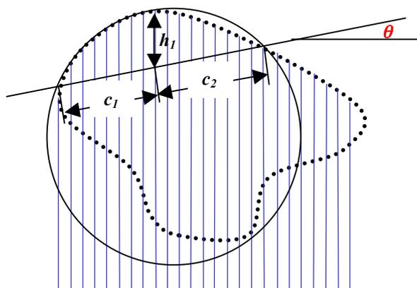
**Figure 4: Dimensions from the profile image of each particle and its reconstituted circle**
