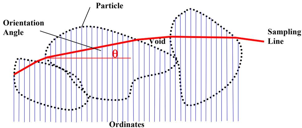
**Figure 3: Detail of the particle train and the sampling line**
