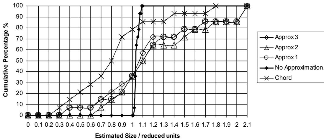
**Figure 6: Size curve showing the relative performance of the reconstituted circle model, its approximations and the original chord size distribution**
