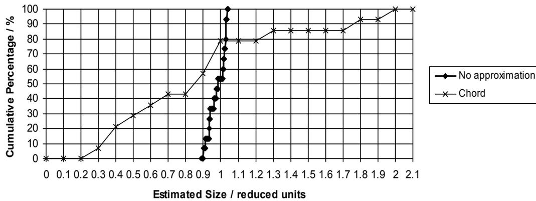
**Figure 8** Size curve showing the relative performance of the reconstituted circle model, with closely-sized particles (0.9 to 1.0 reduced units)
