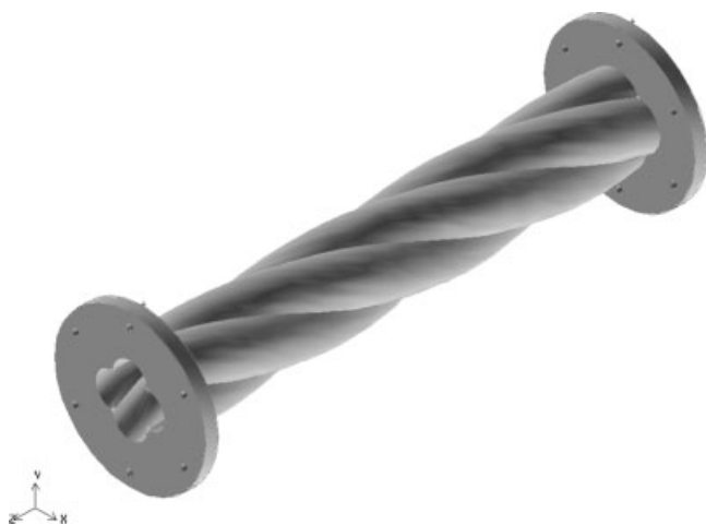
Figure 1. Optimized swirl pipe geometry as determined by previous researchers.
